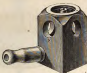
FIG. 66.—Base of ordinary form of Bunsen's burner, showing holes to admit air.
